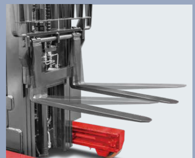
Forks can tilt forward/backward for easy loading
